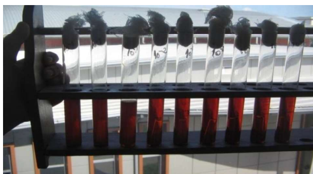
Figure 1. Durham tubes with BGBL medium for the determination of coliform bacteria in milk (personal archive photo)
