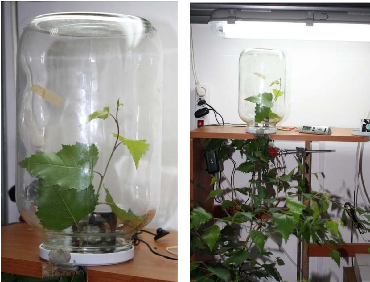
**Figure 1.** Custom-built system for measuring volatile organic compounds
