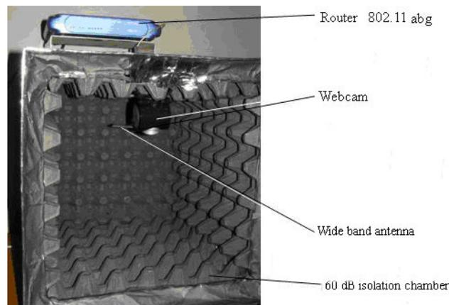
**Figure 1.** Installation to stimulate the plant development by applying a low power electromagnetic field.
